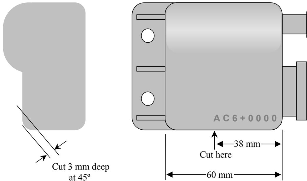
1. Make a 3mm deep cut with a hacksaw in the position shown. Then fill the slot with silicon.
